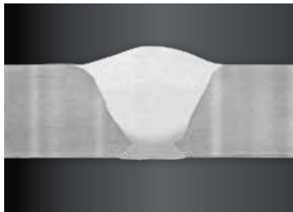
IAC root pass welded in vertical downwards position in 10 mm mild steel; filled with two Sequence Repeat passes in vertical downwards position.
