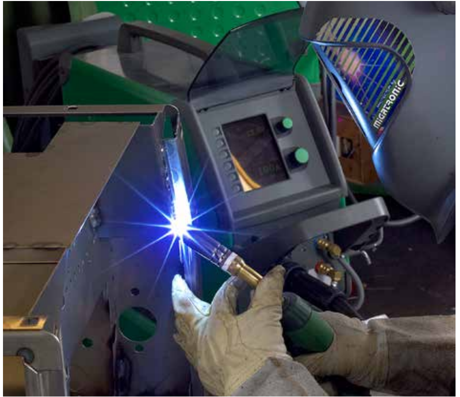
A powerful computer adjusting the process 50,000 times per second is incorporated in the Sigma Galaxy.
