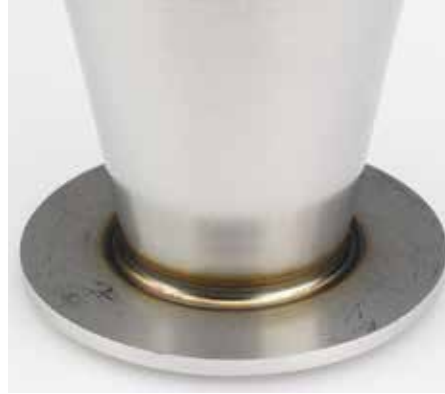
Stainless steel – Plasma-keyhole welding in 6 mm wall thickness
